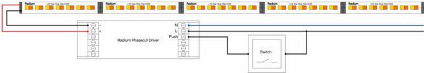
Wiring diagram Radium Phasecut driver in combination with LED Strip WarmDIM
